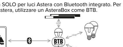
Please power on the BT. Hold down the power button for 3 seconds until the blue light begins to flash. In the AstraApp, "Manage Bluetooth Bridges", then "+" and follow instructions on screen to connect. The light which is connected as BT shows a small Bluetooth icon in the display.
