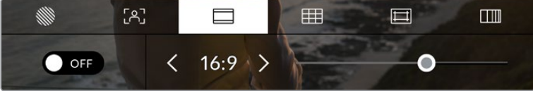
Tap the 'frame guides' icon while accessing 'LCD monitor options' to access your frame guide settings
