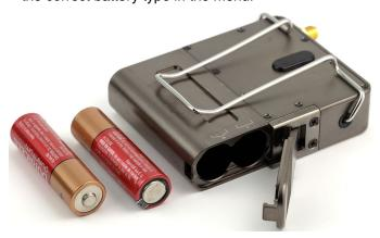
Because rechargeable batteries run down quite abruptly, using the Power LED to verify battery status will not be reliable. However, it is possible to track battery status using the battery timer function available in the receiver.
