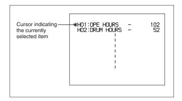
If the SET/MENU button is pressed while holding down the SHIFT button to display the menu settings in the time data display area, a full-screen version also appears on a monitor connected to the COMPOSITE (SUPER) output connector, SDI (SUPER) output connector (J-10SDI/30SDI only), or LDV connector as shown in the above figure.
