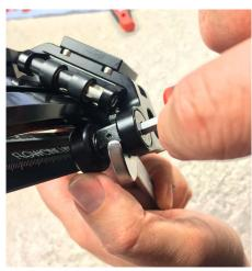
5. After finding the bearing that is too loose (rotating freely without and contact to the bow), take the wrench, and loosen the M8 flat head flowcine screw a little until you can move the shaft.
