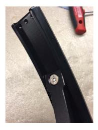
8. Be sure to check the flat heads under each bow so they are tight. If not add some loctite and tighten them again. These are also getting tremendous amount of vibration.
