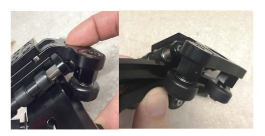
4. Generally, a dot that points inward to centre (left image) will be too loose, and a dot pointing outwards (right image) is too tight. This is highly individual to each bow though. But rotating the dot on the hexagon shaft inwards brings the bearing closer to the bow, and vice versa.
