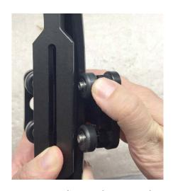
2. Separate the two bows. And turn the bow around and with the thumb check each of the outer roll bearings. IF you can freely roll it, its too loose and you need to tension it. IF you cannot rub it at all, it might be too tight and cause friction. Perfect fit is when you can roll it with your thumb but its still with a bit of friction against the bow.
