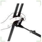
To open the spreader, press the ratchet pin and pull the leg outwards to the desired click stop.
