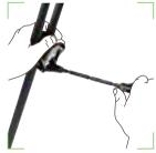
To close, simply push the tripod leg inwards; the telescopic spreader will retract automatically.
