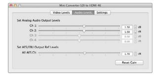
Adjust audio levels using Blackmagic Converter Utility.
