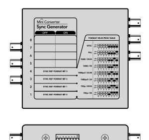
Change your converter's internal settings by adjusting the mini switches using the tip of a pen.
