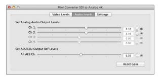
Adjust audio levels using Blackmagic Converter Utility.
