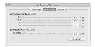
Adjust audio levels using Blackmagic Converter Utility.
