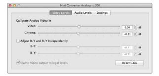
Adjust analog video levels using Blackmagic Converter Utility.
