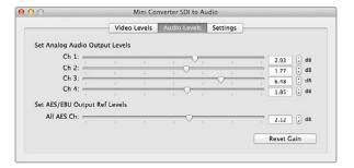
Adjust audio levels using Blackmagic Converter Utility.
