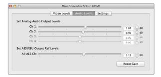
Adjust audio levels using Blackmagic Converter Utility.
