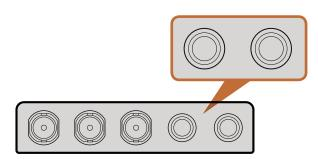
Connect external analog or digital audio to your converter's TRS audio connectors.
