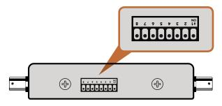
Internal settings are applied by adjusting mini switches with a pen.
