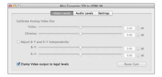
The Clamp Video output to legal levels setting is checked by default. This setting ensures your analog output is a true representation of the SDI input. Adjusting video levels may result in illegal colors.
