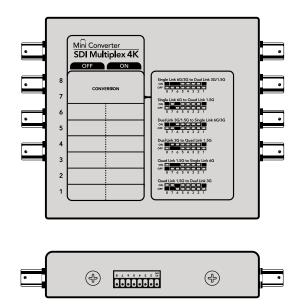
Change your converter's internal settings by adjusting the mini switches using the tip of a pen.
