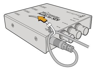
Locking the power cable to the converter's cable tie point prevents accidental disconnection.
