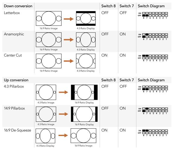
You've probably noticed switches 8 and 7 share settings for up and down conversions. This is because aspect ratio settings are determined by the output settings. For example, if you have switches 3 and 2 set for 1080i50 HD output, and processing switch 1 set to ON, Mini Converter UpDownCross will automatically set switches 8 and 7 for down conversion.
