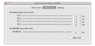
Adjust audio levels for the selected analog channels or AES/ EBU audio reference levels using Blackmagic Converter Utility.
