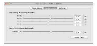
Converter Utility can be used to adjust audio levels.
