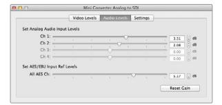
Adjust audio levels using Blackmagic Converter Utility.
