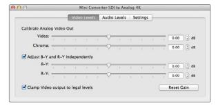
Adjust analog video levels using Blackmagic Converter Utility. The Clamp Video output to legal levels setting is checked by default. This setting ensures your analog output is a true representation of the SDI input. Adjusting video levels may result in illegal colors.
