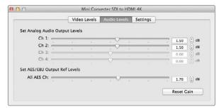
Adjust audio levels using Blackmagic Converter Utility.
