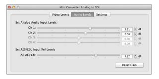
Adjust audio levels using Blackmagic Converter Utility.
