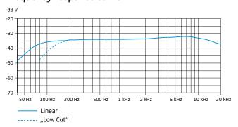
The original measurement protocol is included with each microphone, measured from 50 to 20,000 Hz.
