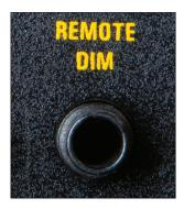
Insert the dimmer cable into the receptacle marked **REMOTE DIM**.
