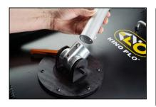
The Mount fittings are U.S. industry standard "Speed Rail" 1 1/4" fittings. They accept a 1 5/8" outside diameter pipe.
