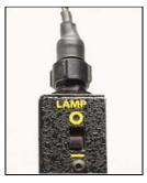
**4)** Turn on power switch, "I", on ballast after power is applied.
