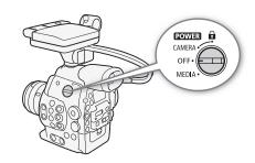
To turn off the camcorder Set the **POWER** switch to OFF.
