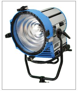
The lamphead is equipped with a CCL module (compensation for cable loss). When operated with the ARRI EB 2.5/4 kW HS AutoScan with CCL, full power is maintained all the way to the lamp even when very long cables are used. This means uniformly high light output indepent from cable length.
